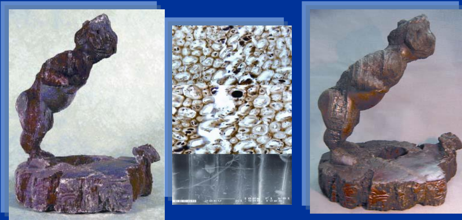
Artefact (Mexico) in poor condition (L) restored by polymeric reinforcement (c) using radiation technology to make it an 'as good as new' piece (R)
